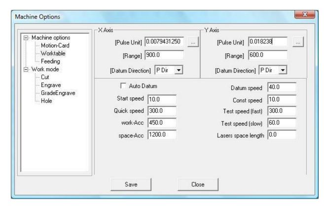
10) Change the value for the Y-Axis [Pulse Unit] to 0.01823829. This is the "approximate" value for the drive end of the rotary axis. This number might be different depending on the diameter of the O-rings in your rotary attachment.
