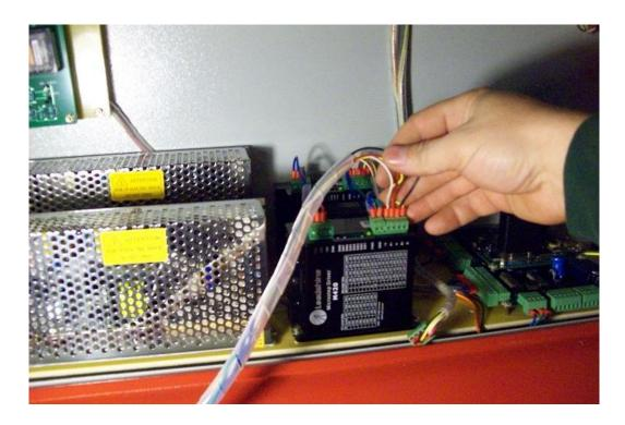
\*\*\* Make sure the power is OFF before you remove the motor wires. Tie the wires off to the side. Place the wire connector (for the rotary attachment) onto the connector of the Y-Axis amplifier. Do not push too hard... It helps to slightly wiggle the connector as you push it on. After everything is reconnected, turn the power back on.\*\*\*
