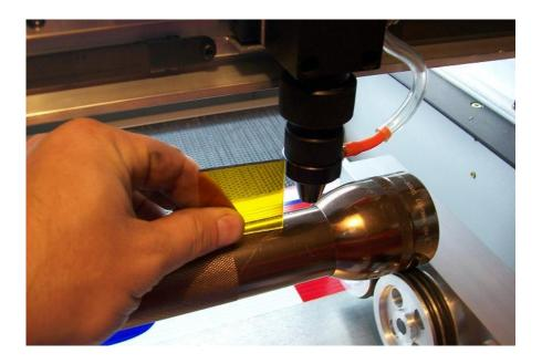
4) Now to make sure the laser will be in focus. Move the focal assembly to the right end of the material and bring the worktable up to make a focused position. Be carefull not to run the material too far up.
