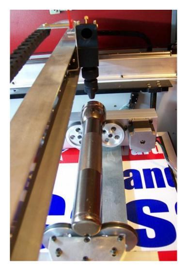
3) Look at how the rotary attachment sits under the Y Axis Rail. Align the rotary attachment to be in line with the rail. We need for the laser to hit in the "top-dead-center" of the material that you have on the rotary attachment.
