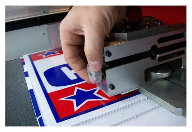
\* This picture shows the knob for adjusting the height of the tail-stock end of the rotary attachment.
