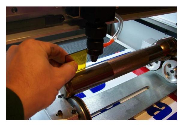
5) Move the focal assembly to the tail-stock end of the material and adjust the rollers up to make a focused position. Be carefull not to run the material too far up. The flashlight in this picture will have a long distance that could be engraved, but some materials may only present a short distance that could be in focus.. (example: short wine glasses)
